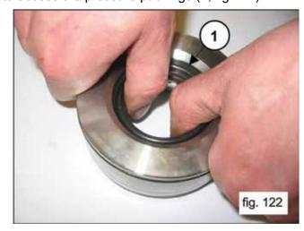
To remove the low pressure packing, use a shim or another tool that doesn't damage the seat of the packing support (1, fig. 123).
