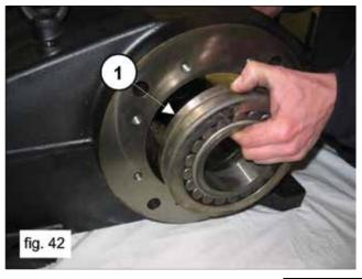
Insert the shaft (1, fig. 29) until the pre-assembled bearing is aligned with the edge of the crankcase (1, fig. 43).
