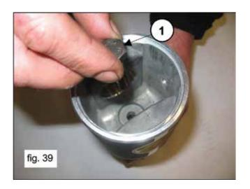
Block the rod using a clamp, and proceed with calibration using a torque wrench (1, fig. 40) as indicated in paragraph 3. "SCREW CALIBRATION"
