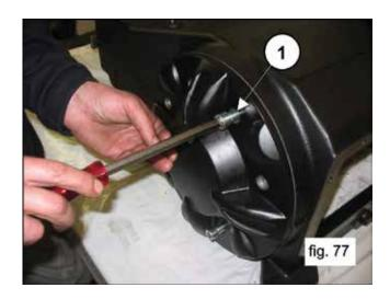
Complete the assembly of the crank mechanism by applying the plugs and lifting eyebolts with the related sealing O-ring.
