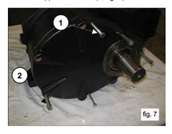
Screw on the 3 threaded screws (1, fig. 8) and simultaneously, using the appropriate tool (p/n F27516700), hammer on the tool itself so that the bearing remains on the pinion when extracting the cover (1, fig. 9).
