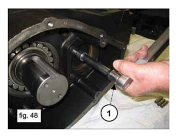
Completely insert the pressure sleeve on the shaft from the opposite side of the PTO (1, fig. 49 and fig. 50).
