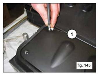
Calibrate the screws with the torque wrench as indicated in paragraph 3. "SCREW CALIBRATION"
