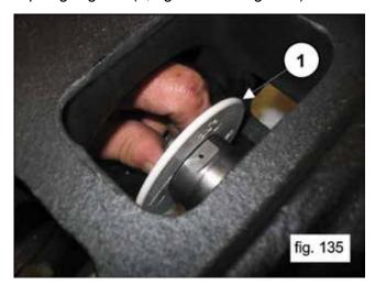
Insert the 14 x 2 O-ring in its correct seat on the plunger bolt (1, fig. 136).
