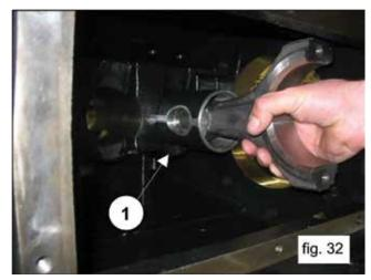
Couple the connecting rods with the previously disassembled caps; be sure to respect numbering (1, fig. 33).
