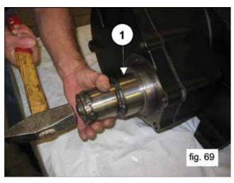
Insert the oil seal inside the reducer flange using the proper tools, p/n F27515900 and F27548200 (1, fig. 70). Before proceeding with oil seal assembly, verify the conditions of the sealing lip. If replacement is necessary, position the new ring as indicated in fig. 71.
